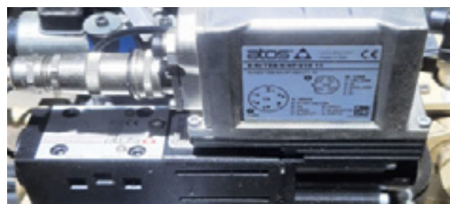
AFTER MODIFICATION- SERVO VALVE ARRANGEMENT FOR UNIT AUTOMATION
